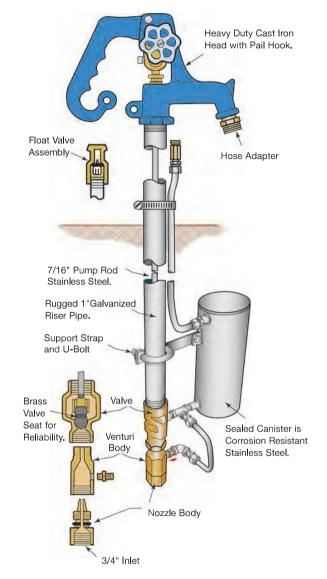
The Brass Packing Nut located on the head of the Simmons Sanitary Yard Hydrant has been factory adjusted. If leakage should occur upon installation or after usage, you may find it necessary to slightly tighten the Brass Packing Nut.
